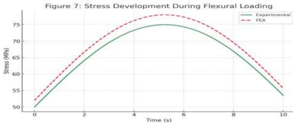
Figure 7: Stress development over time during flexural loading for both experimental and FEA approaches. The graph illustrates the progression of stress as the composite undergoes bending deformation, highlighting consistent peak stress behavior and waveform alignment between the two methods.
