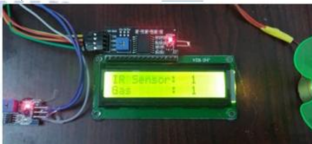
Figure 5 LCD display for IR sensor and GAS sensor
