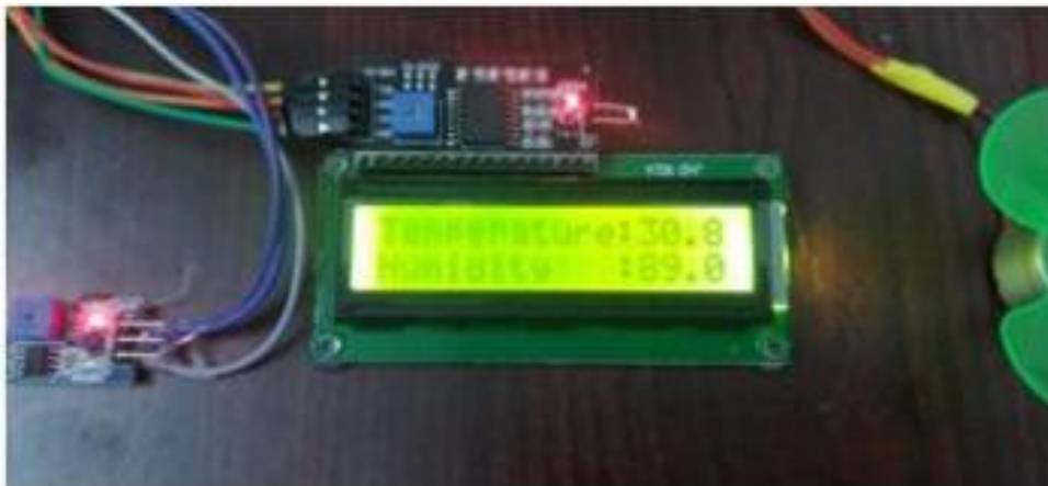
Figure 4 LCD display for temperature and humidity sensor
