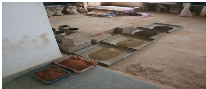
Figure 1: Preparation of soil sample for testing.
