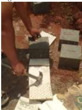
Fig.4 Demolding of translucent concrete cubes
