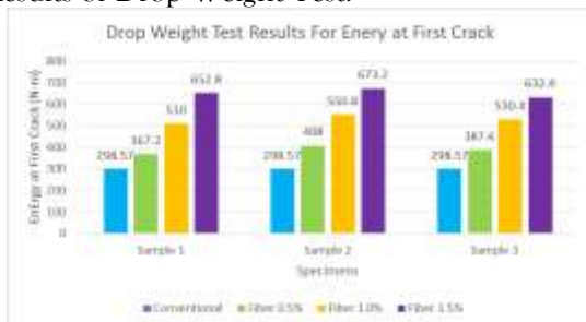
Fig.11 Drop Weight Test Result for Energy at First Crack
