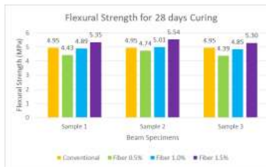
Fig.8 Flexural Strength for 28 days curing
