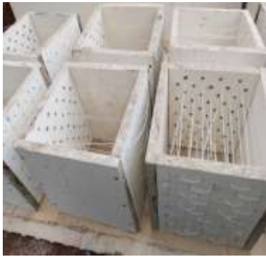
Fig.2 Moulds fabricated for Concrete cubes.
