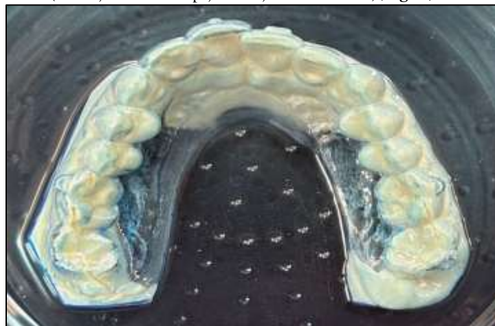
Figure 6: 1.25mm model showing visible deformation after thermoforming
