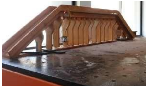
Figure-7 Wooden Bridge on Shake table
