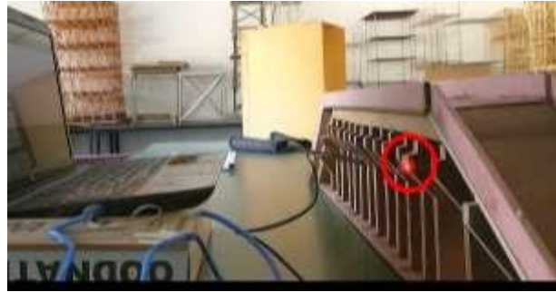
Figure-1 Accelerometer Sensor on Bridge
