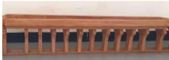
Figure-2 Bridge scaled model
