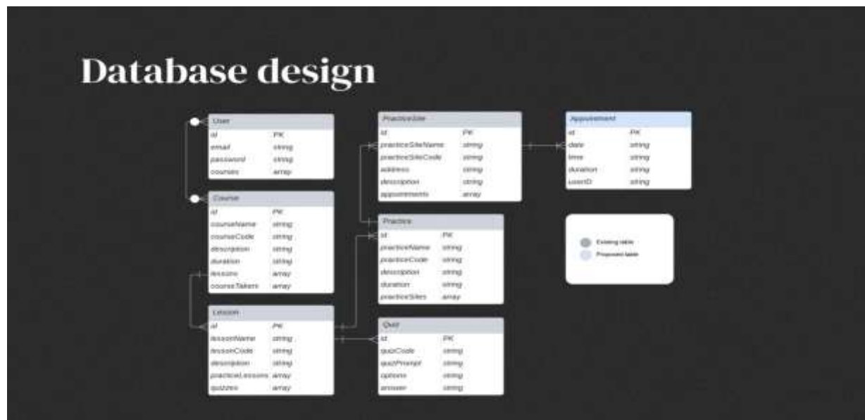
Figure 6. Database design used for the MVP with models and their relationship
