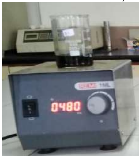
Fig. 1 Magnetic Stirrer used for mixing of nanofluid
