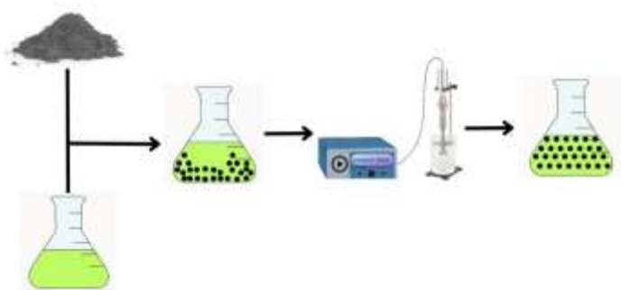
Fig. 6 The preparation process of ethanol glycol based nanofluid.
