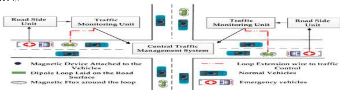
Fig 1. Layout Architecture for Efficient Dynamic Traffic Control System
