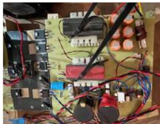
Figure 22 (a) : Two-wheeler EV charger hardware circuit with pfc, controller driver circuit and Figure (b) Hardware assembly of experimental set up (prototype EV charger)
