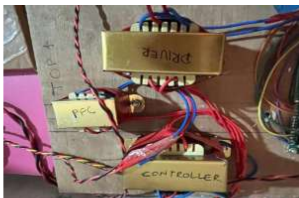
Figure 22 (a) : Two-wheeler EV charger hardware circuit with pfc, controller driver circuit and Figure (b) Hardware assembly of experimental set up (prototype EV charger)
