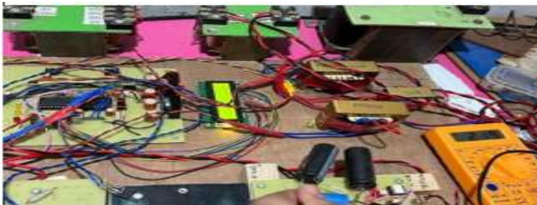
Figure 21: Two-wheeler EV charger experimental set up (hardware prototype circuit)
