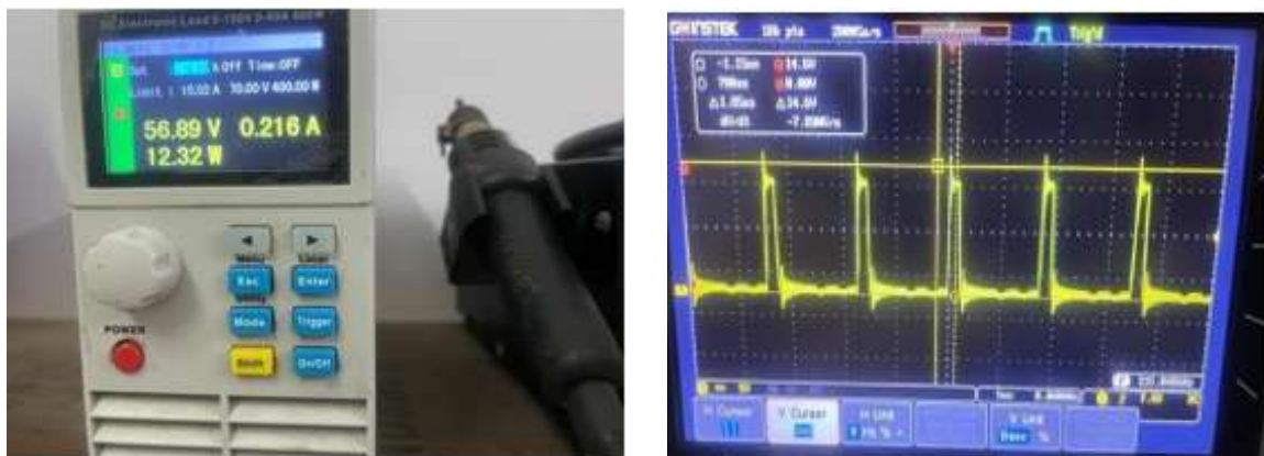
Figure 26: (a) IGBT waveforms at different loading conditions
