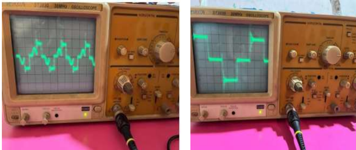
Figure 24: Switching waveforms of IGBT under off and on load conditions
