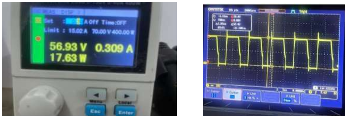
Figure 27: (b) IGBT waveforms at different loading conditions from no load to full load condition
