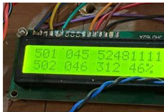
Figure 23 (c): LCD Display Module Showing Real-Time Charging Parameters for an Improved Two-Wheeler Electric Vehicle Battery Charger and Figure (d) Close-Up of LCD Display Showing Detailed Charging Metrics in Real-Time Parameters for a Two-Wheeler Electric Vehicle Battery Charger
