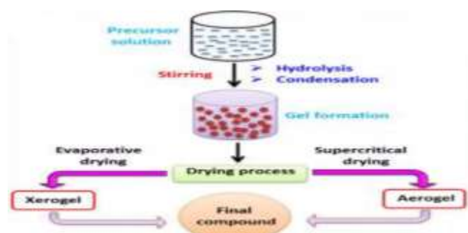
Fig 1 Steps of the Sol-Gel method
