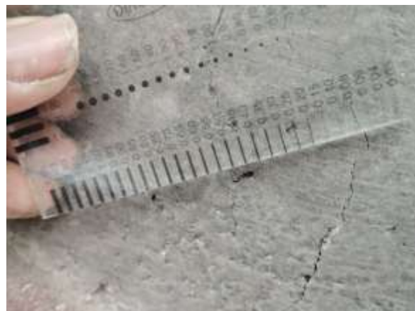
Figure 9 (b): Photo showing of crack and crack width measurement
