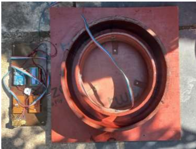
Figure 2: Photograph of ring specimen and data acquisition system
