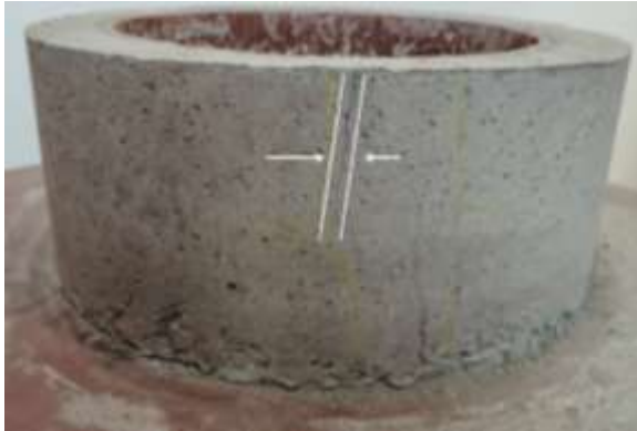
Figure 11 (a): M60 concrete cracking
