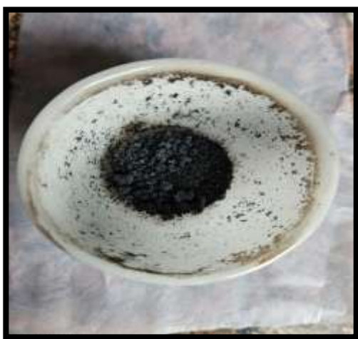
Fig 1 Crucible not fully ignite and not became colorless
