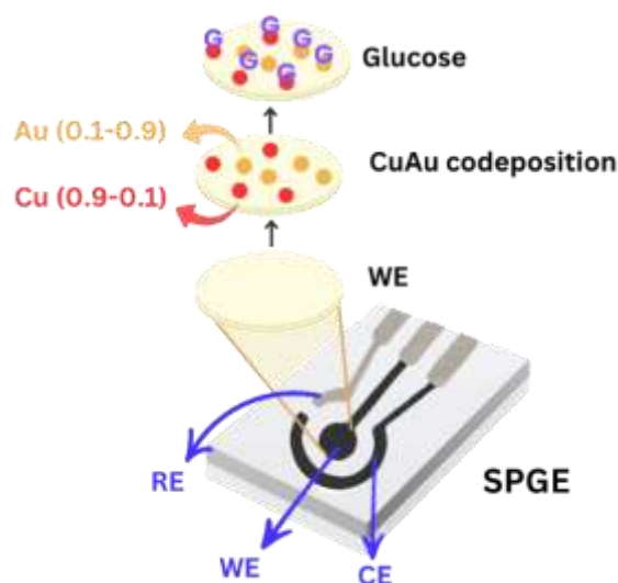
Figure 1. Schematic of Au-Cu co-deposition on SPGE for glucose detection, with varying Au:Cu ratios (0.1–0.9) modifying the working electrode (WE).
