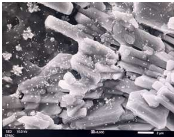
Figure 2 SEM image of Au-Cu codeposition on SPGE (6,000x magnification), showing a porous Cu matrix with dispersed Au nanoparticles. Scale bar: 2 \mu\text{m} .
