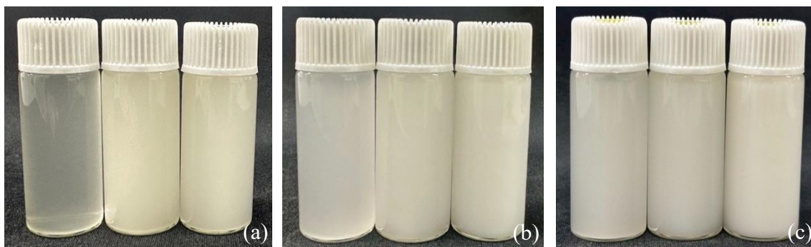
Figure 5: Shows nano emulsions in the ratio between oil (% w/w) and surfactant (Tween 80 + Span 80) (% w/w), where (a) = green bean oil, (b) = soybean oil, and (c) = red bean oil.
