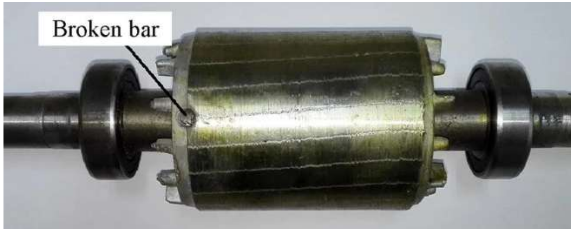
FIGURE 2. Faults in broken rotor bars result in speed oscillations within the rotor, leading to accelerated wear of the bearings.
