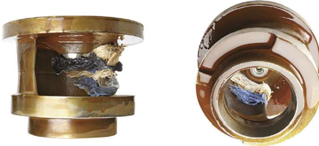
FIGURE 5. A clogged impeller diminishes the efficiency of the pump. This condition can be artificially induced by utilizing polystyrene to obstruct the impellers.
