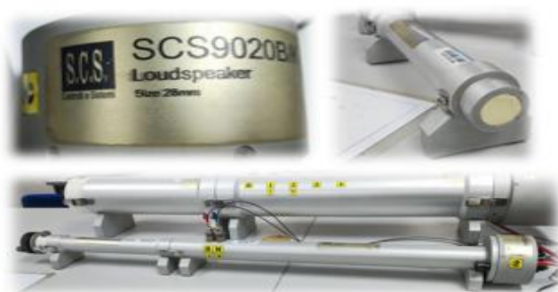
Figure 2. Acoustic impedance tube test setup used at UTHM (Model SCS9020B/K).
