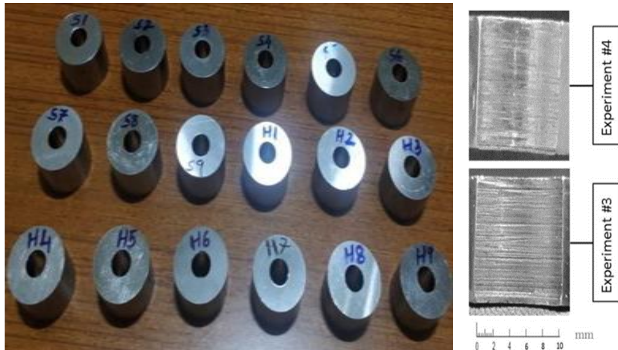
Fig 2: Surface topography of machined holes.
