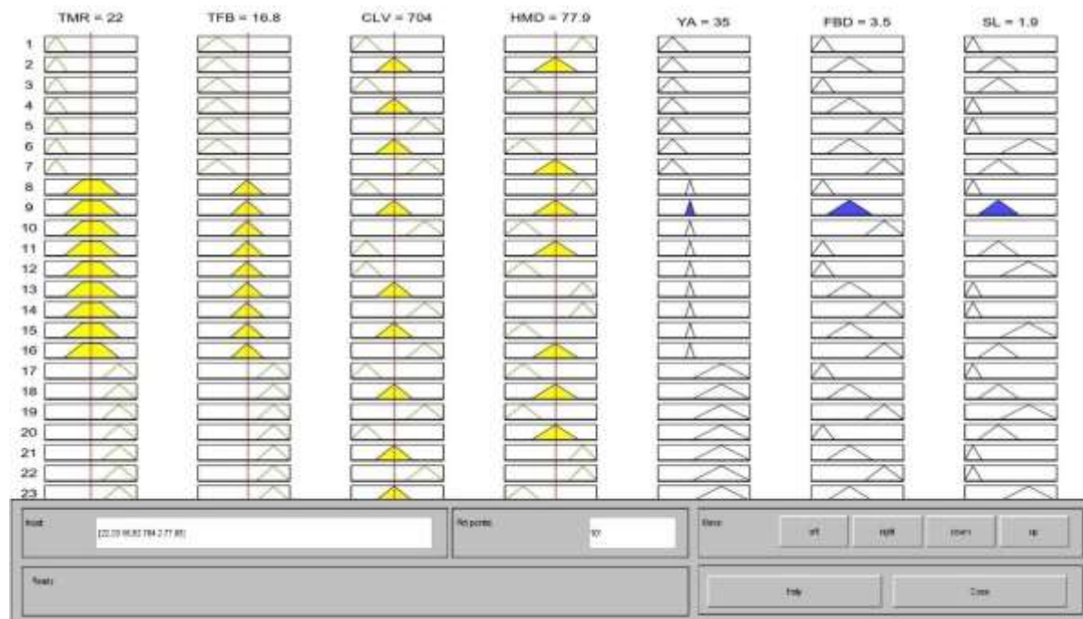
Figure 4 Evaluation of the rule for button mushrooms with medium yields and medium quality The fuzzy rule evaluation for button mushrooms under environmental conditions, which yields a medium yield and quality, is shown in Figure 4. The diagram illustrates how the system reacts to input values such as TMR = 22, TFB = 16.8, CLV = 704, and HMD = 77.9 using MATLAB's Fuzzy Logic Toolbox. The active membership levels for the inputs across linguistic phrases such as Low, Medium, and High are indicated by the yellow shaded zones. The ensuing fuzzy outputs for variables such as stalk length (SL), fruiting body diameter (FBD), and yield amount (YA) are shown by the blue areas. This demonstrates how well the system maps environmental elements to agricultural outputs and how interpretable it is.
