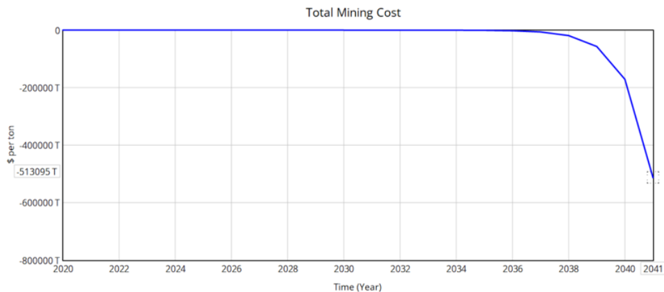
Fig. 15 Scenario simulation 5 results. System Dynamic study simulation at reduction of underground block cave production capacity (exclusion of high pyrite areas) with additional modification of ore processing facility and sedimentation pond in overcoming pyrite contamination issues. Scenario 5 presenting trend decline in total mining cost at lesser value compared to scenario 4.
