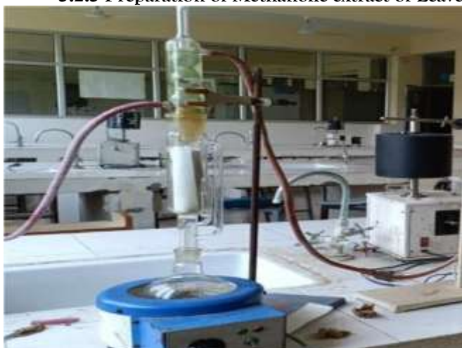
Figure no 3: Extraction of Rubus ellipticus by Soxhlet apparatus
