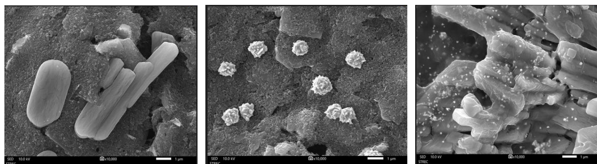
Figure 2 SEM images of (a) Cu-modified SPGE (Cu/SPGE), (b) Au-modified SPGE (Au/SPGE), and (c) Au-Cu co-deposited SPGE (Au-Cu/SPGE) at a magnification of 10,000X.
