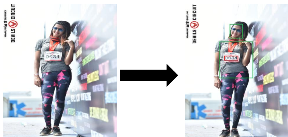
Fig 8. Detecting face, estimating torso and localizing Bib/Jersey number location
