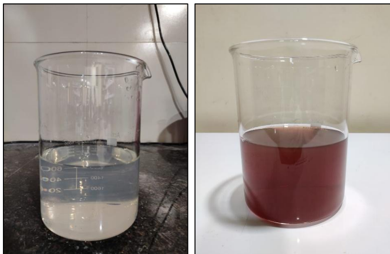
Figure: Color change from colorless to dark brown confirms the synthesis of silver nanoparticles
