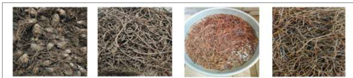
Fig.2.1. Extraction of fibres from Curcuma longa roots by using the water retting method
