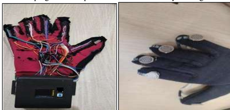
Figure 4: Prototype of smart rehabilitation glove for brain stroke patients
