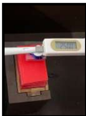
Fig.2: Standardized brushing force of 250 g applied using a force gauge
