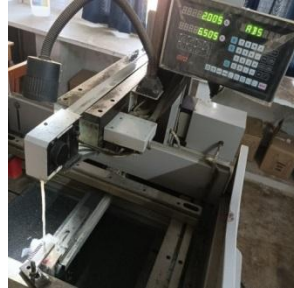
Figure 03 (a) CNC WEDM Figure 03 (b) Processing of Specimen on setup
