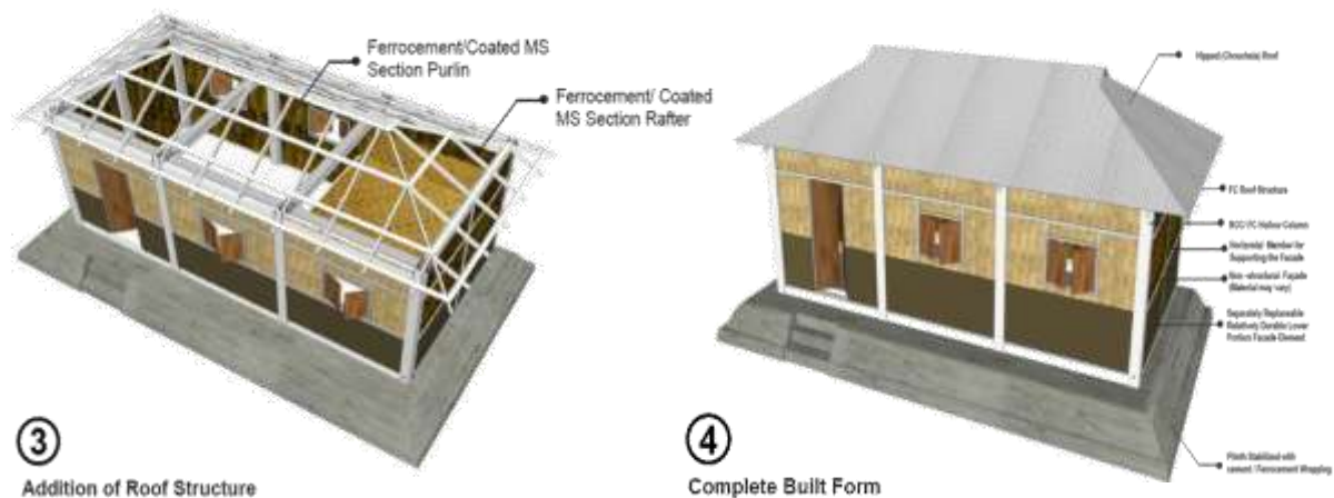
Figure no 7: Upper structure formation of house module
