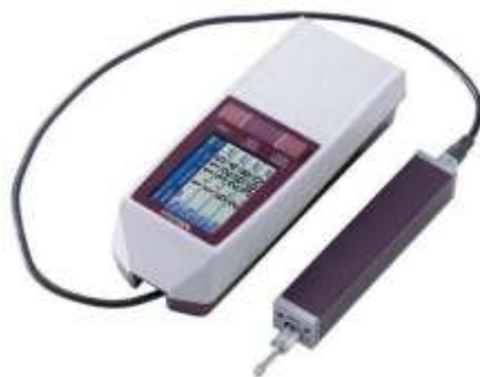
Fig.4. Surface Roughness Tester Mitutoyo
