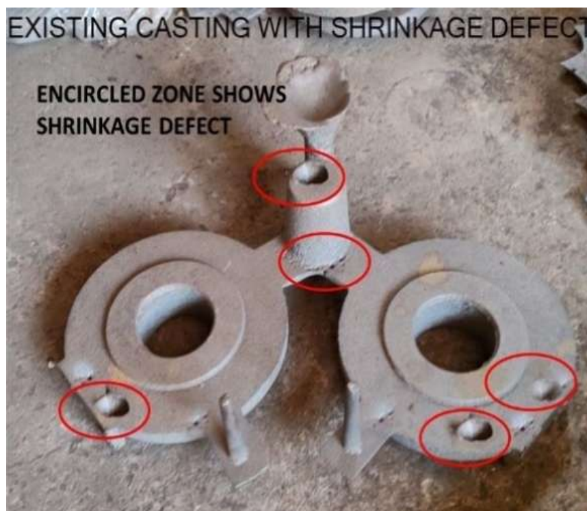
Figure 1 Shrinkage defect in casting
