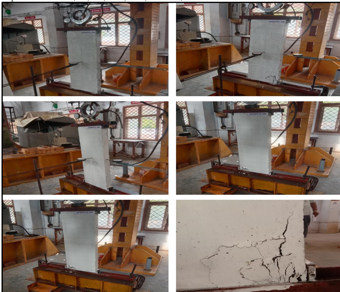
Figure 9: Failure pattern of wall panels
