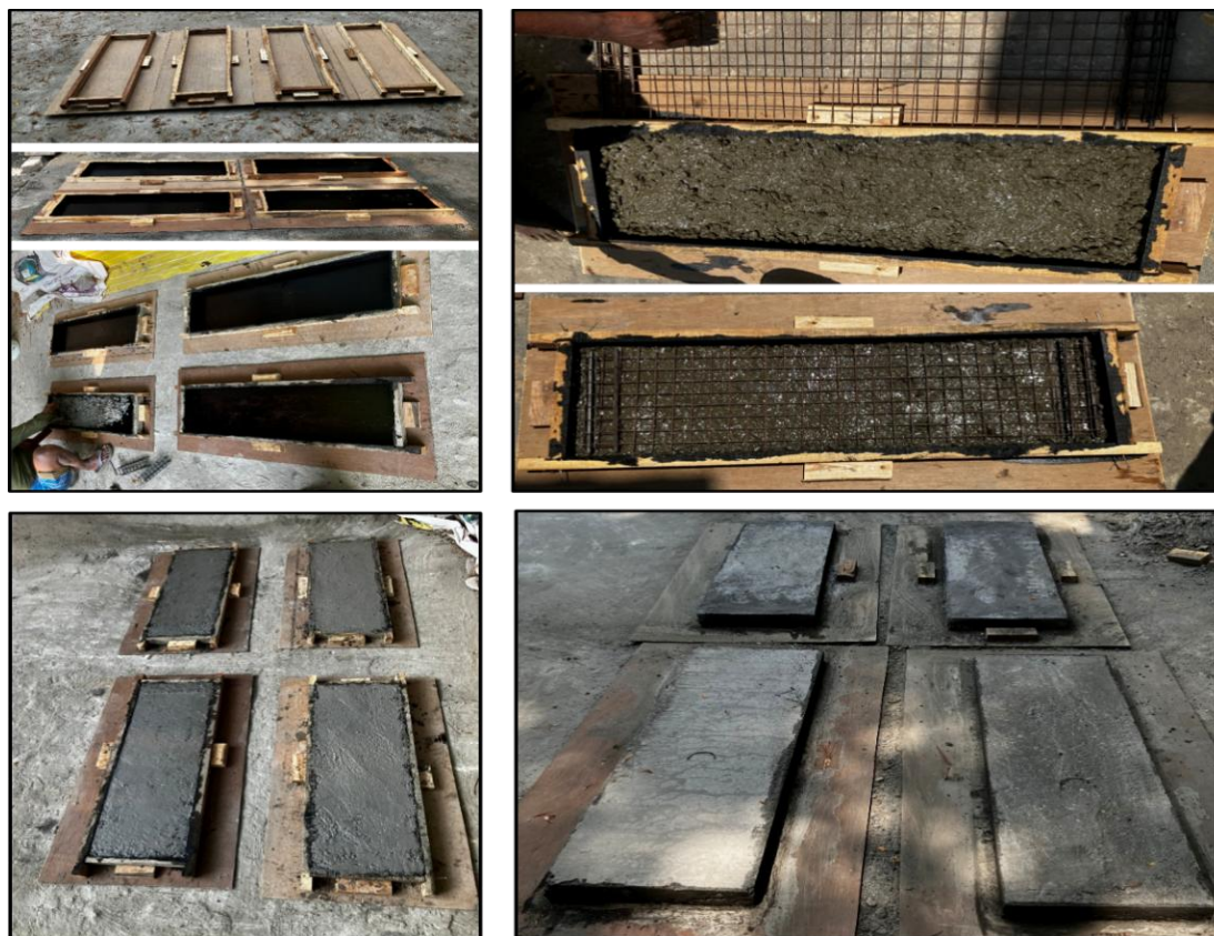
Figure 5: Wall panels preparation setup and prepared wall panels
