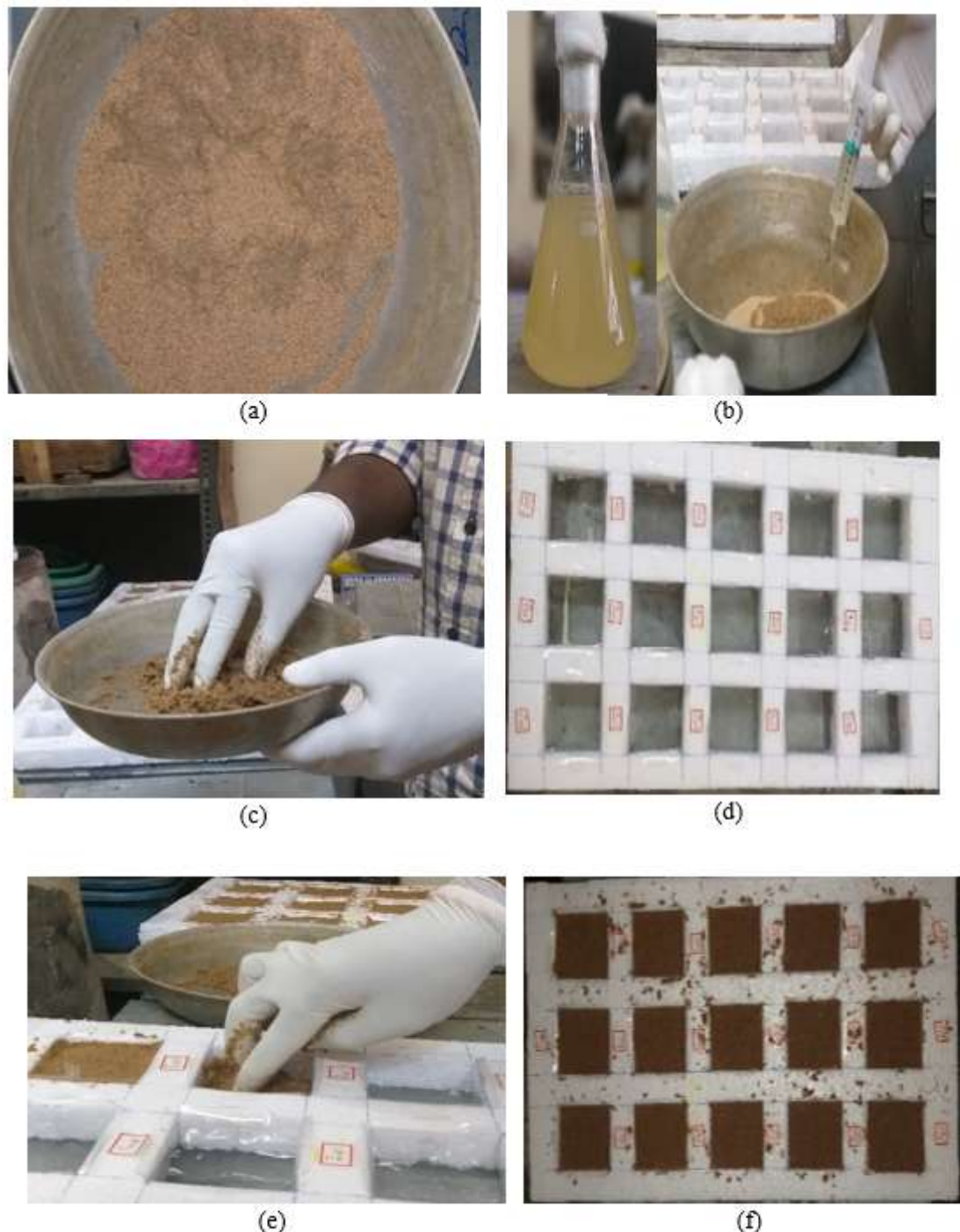
Figure 5: Sample Preparation for Testing; (a) Sand-Coir fiber Mixture; (b) Adding Bacteria Solution to Soil-Fiber Mix; (c) Mixing Sample for Uniformity; (d) Mould; (e) Placing Samples in mould; (f) Curing of Samples
