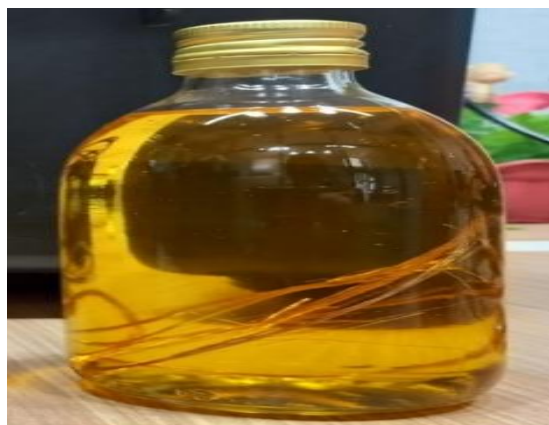
Figure 10. 100% flaxseed oil that has been heated for 5 hours with a copper bath.
