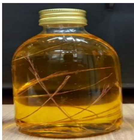
Figure 11. Mixing 50% Flaxseed Oil with 50% Coconut Cooking Oil, which has been heated for 5 hours with a copper bath.
