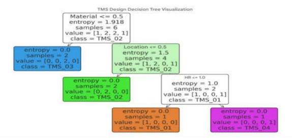
This tree shows the classification logic flow to determine the type of Temporary Modular Shelter (TMS) design based on a combination of category values (Low, Medium, High) of the three factors.
