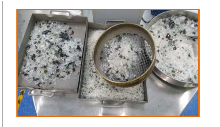
Figure 2: coarse and fine fractions after crushing with the Los Angeles machine: Authors' own.
