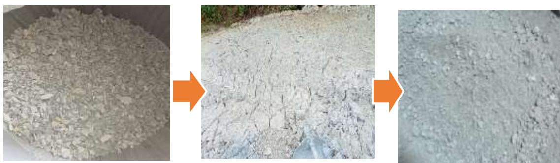
Fig.1 Process of forming Calcium Carbide Residue
