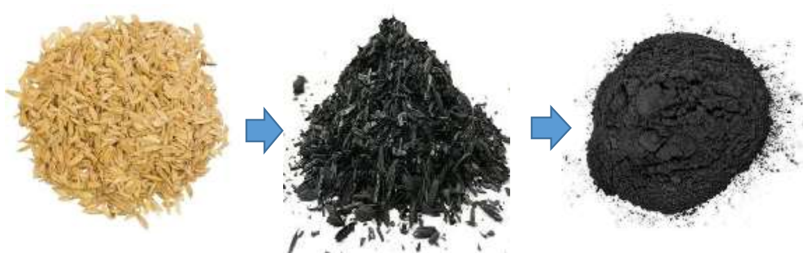
Fig.2 Process of forming Rise Husk Ash
