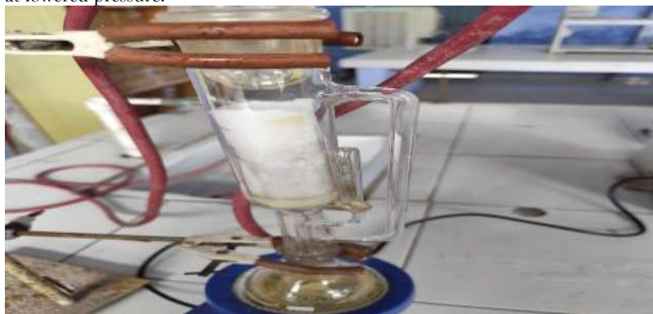
Fig 1: - Soxhlet extraction apparatus used in the preparation of plant extracts for phytochemical analysis.
