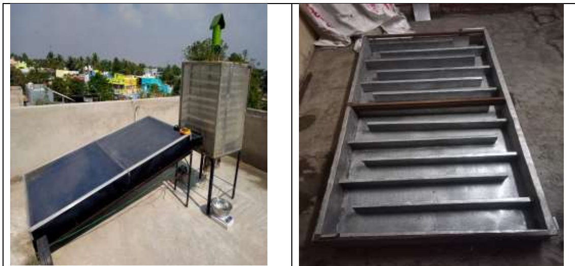
Fig 1. Photograph of the indirect solar dryer with thermal storage and PCM container
