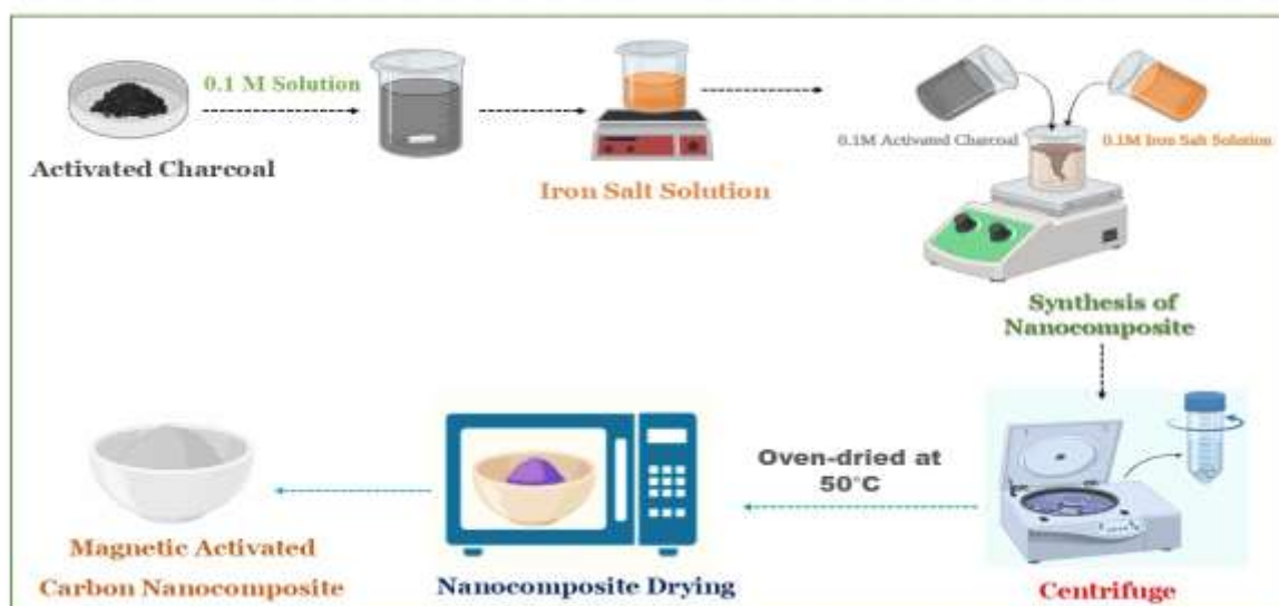
Fig.1 Schematic representation of the synthesis of Magnetic Activated Carbon Nanocomposite.
