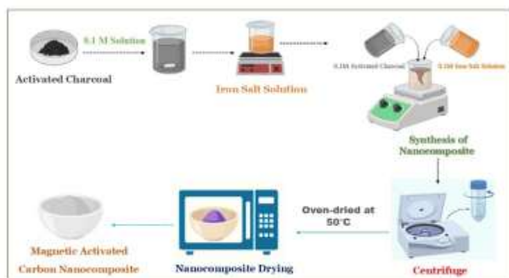
Fig.1 Schematic representation of the synthesis of Magnetic Activated Carbon Nanocomposite.
