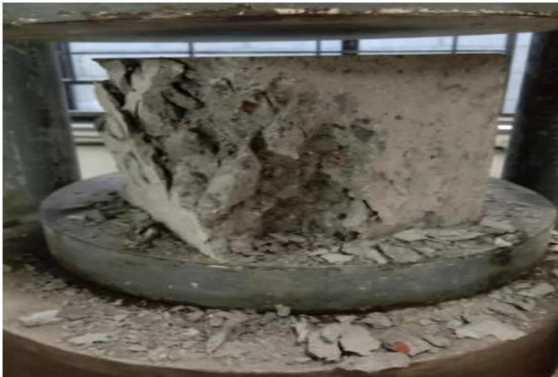
Fig 7 Cube Break after testing
