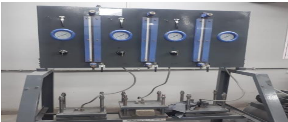
Fig 9 Rapid Chloride Penetration Test setup
