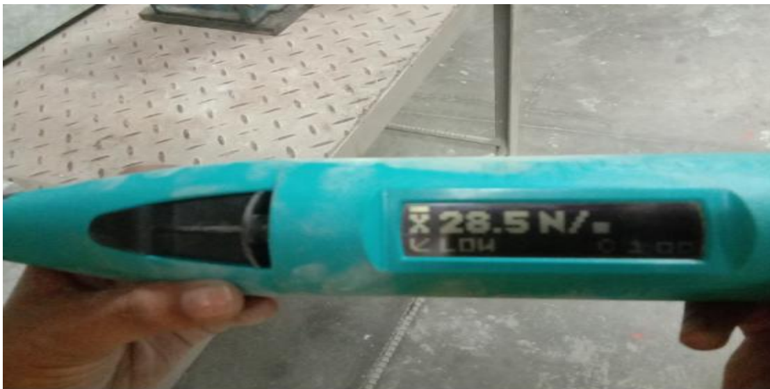
Fig 5 Rebound hammer test on cube
