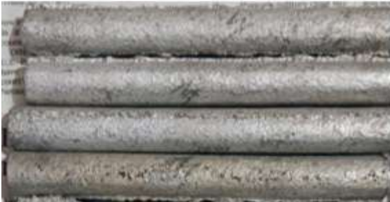
Figure 2: The alloy contains of a foremost epoxy matrix, reinforced with a average percentage of glass fibres and a little amount of aluminium grains to strengthen strength and stiffness
