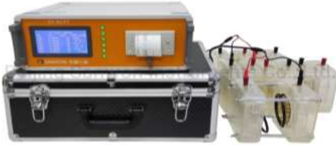
Fig4. Rapid Chloride Penetration Test
