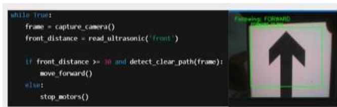
Fig. 10. Forward direction being detected and will move forward accordingly based on the direction showed in the cam feed.
