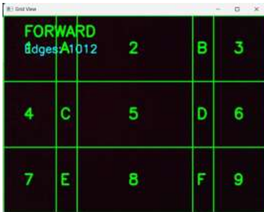
Fig. 7. This figure displays the output of a grid-based path recognition system for an autonomous wheelchair
