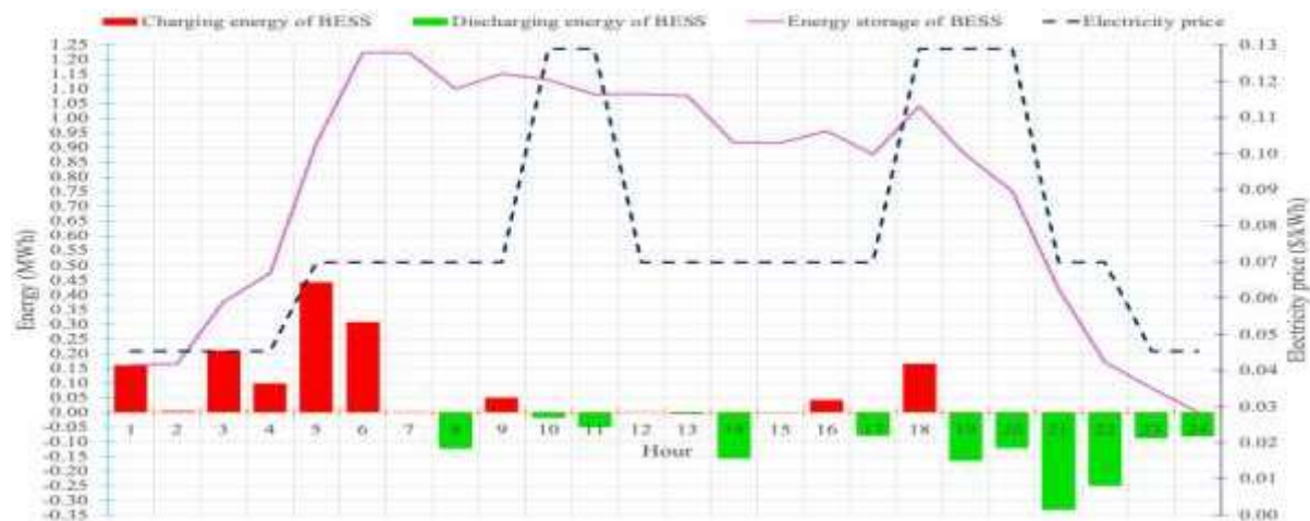
Figure 7. The energy charging and discharging of the BESS at node 33 over 24 hours, along with the corresponding electricity prices
