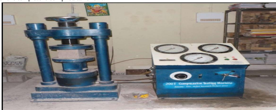
Fig 3 Laboratory compression testing machine setup
