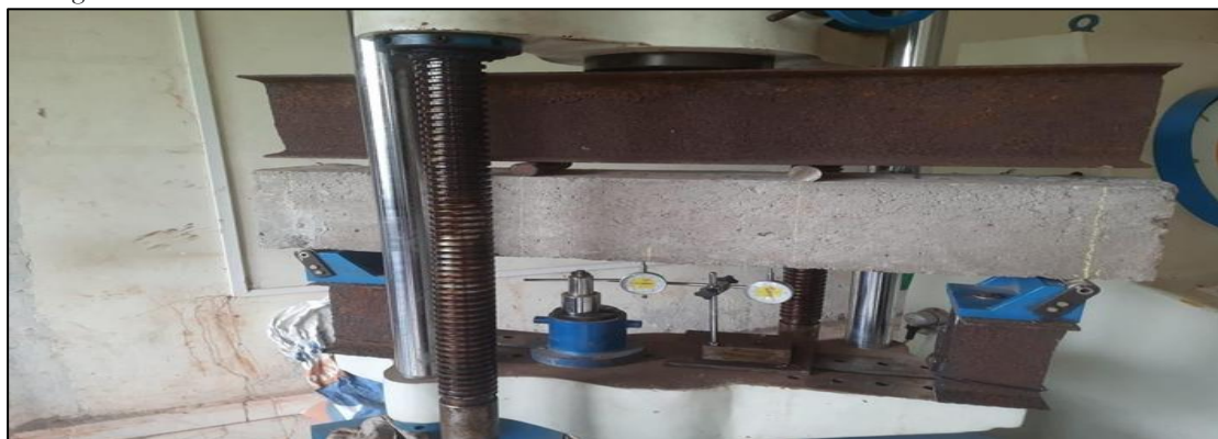
Fig 9 Flexural Strength Test on beam
