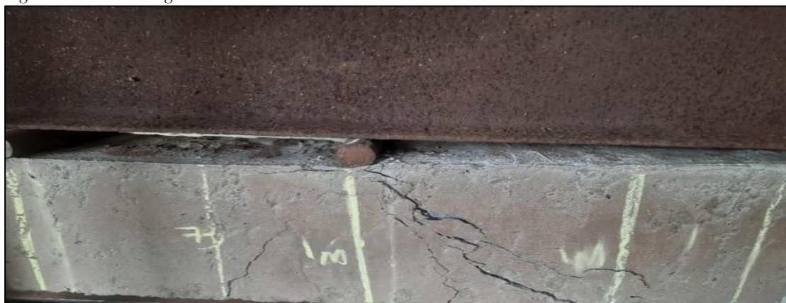
Fig 10 Initial Crack Propagation in Control Beam
