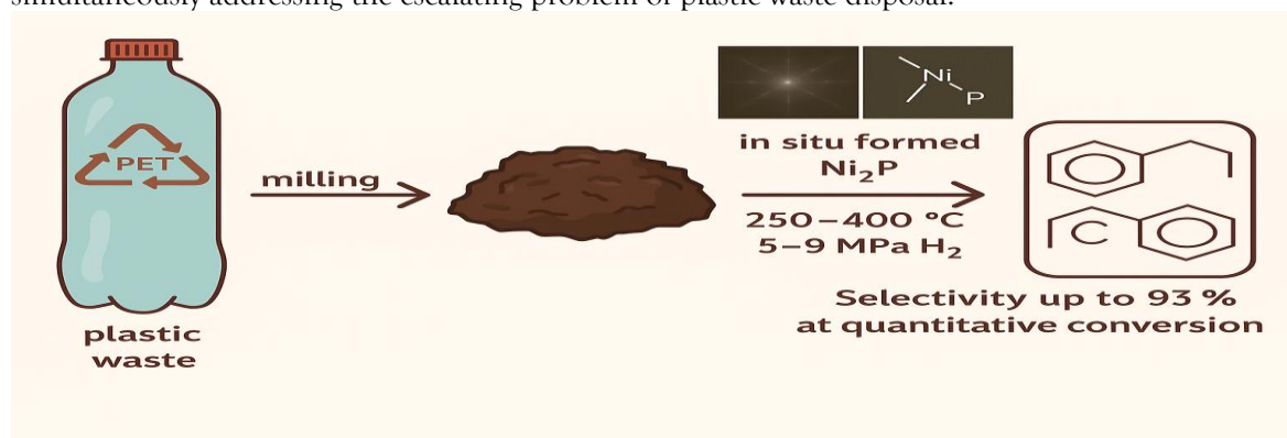
Fig 1: Catalytic Upcycling of PET Plastic Waste into Aromatic Compounds Using In-Situ Formed \text{Ni}_2\text{P} Catalyst
