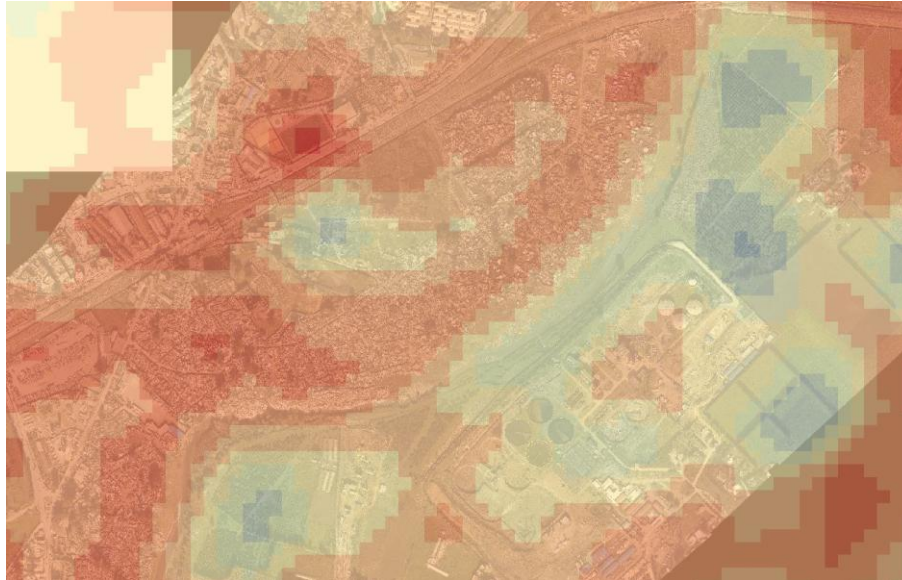
Figure 6. Interpolated TempSensor data on a Quick Bird image background (Algiers, July 23 rd , 2022).
